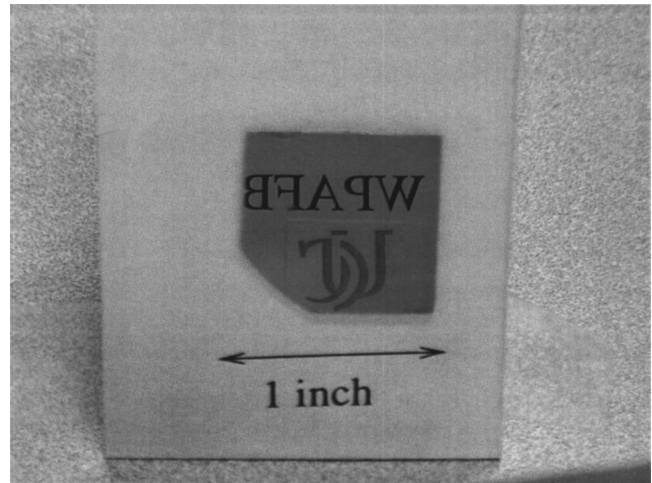
Fig. 1. Photograph of a LaS thin film grown by PLD on a (100) Si substrate. The film appears golden yellow in color with a mirror-like surface morphology, as indicated by the reflection of a logo symbolizing our team effort. The PLD deposition is uniform over a 1 in. square area.
