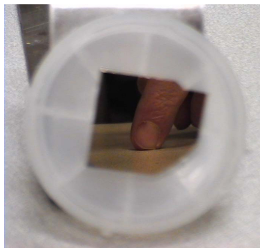
FIG. 5. (Color online) Thin film of LaS deposited by PLD on a square inch Si substrate. The reflection of the finger shows the metallic character of the thin film. [Reprinted with permission from M. Cahay, K. Garre, X. Wu, D. Poitras, D. J. Lockwood, and S. Fairchild, Journal of Applied Physics 99 , 123502 (2006).]
