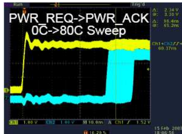
Figure 22 – Sleep to Active latency plot with temperature sweep
